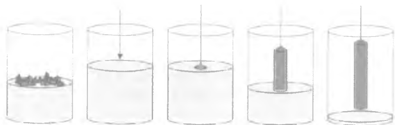
3.9-rasm. Si monokristallini Chochralskiy usuli bilan o'zlash qurilmasining tasviri: 1 – Si zatrovkasi, 2 – Si monokristalli, 3 – SiO 2 qozoni, 4 – Si eritmasi, 5 – grafitli ushlagich, 6 – qizdirgich, 7 – inert gaz (Ar)
