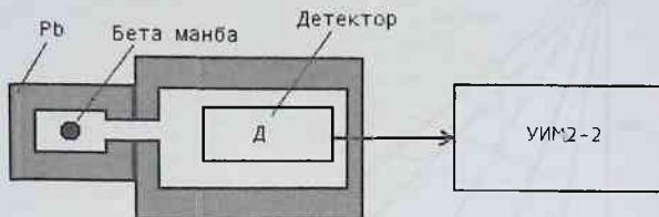
4-rasm. \beta -zarracha manbaining aktivligini o'lchash blok-sxemasi
