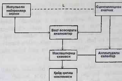
3-rasm. Neytron spektrometrining soddalashtirilgan sxemasi
