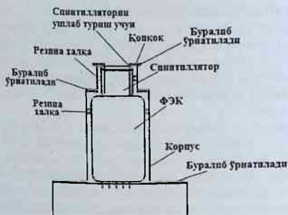
5-rasm. Ssintillyatsion detektorni yig'ish tartibi
