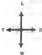
condition at min drag
