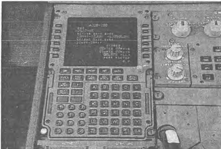
A321 Multipurpose Control & Display Unit (MCDU) Interface to Flight Management System
