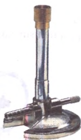
17-rasm. Gaz gorelkalari Bunzen gaz gorelkasi
