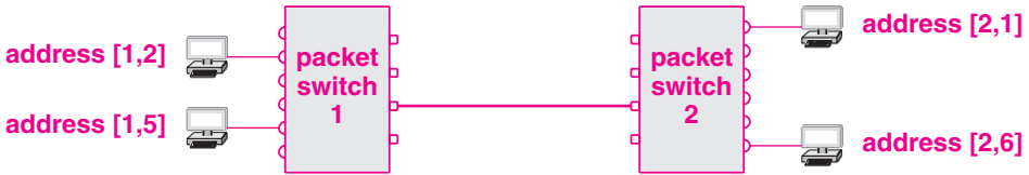
Figure 18.4 Example of an address hierarchy where each address identifies a packet switch and a computer attached to the switch.
