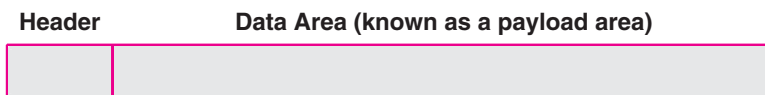
Figure 22.1 The general form of an IP datagram with a header followed by a payload.
