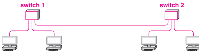
Figure 26.4 Four hosts connected by two switches.
