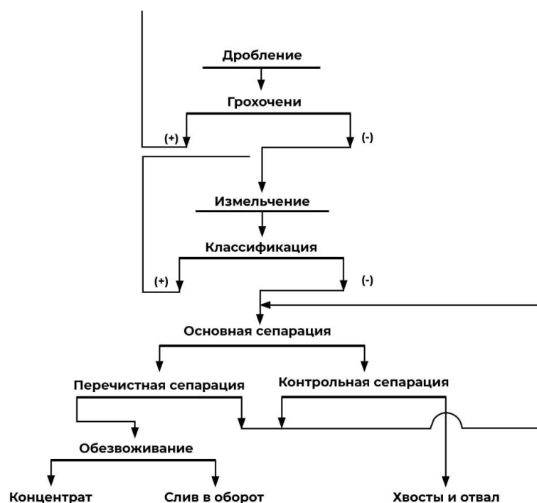
Figure 2.2 - Schematic diagram of mineral processing
