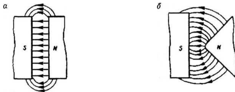
Figure 10.2 - Scheme of a homogeneous (a) and heterogeneous (b) magnetic fields
