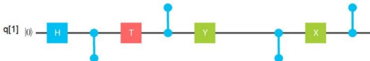
(b) The "bristle-brush" pattern formed by the gates applied to qubit q[1]
